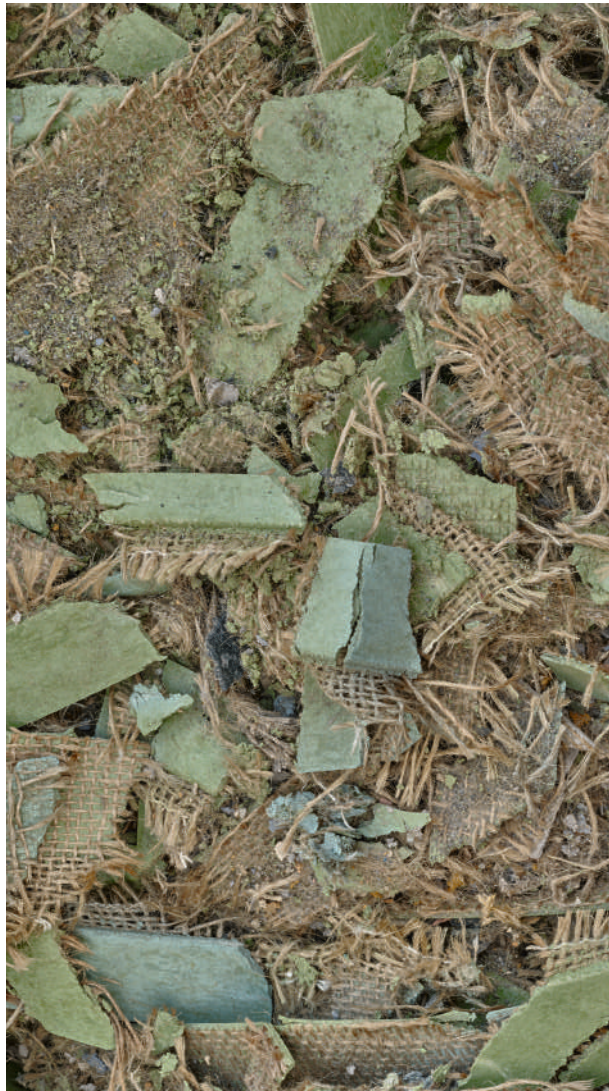
1. Shredded Linoleum Through ReStart®, our innovative take-back and recycling programme, post-consumer linoleum and installation off-cuts are returned to our on-site recycling centre and mechanically shredded.
