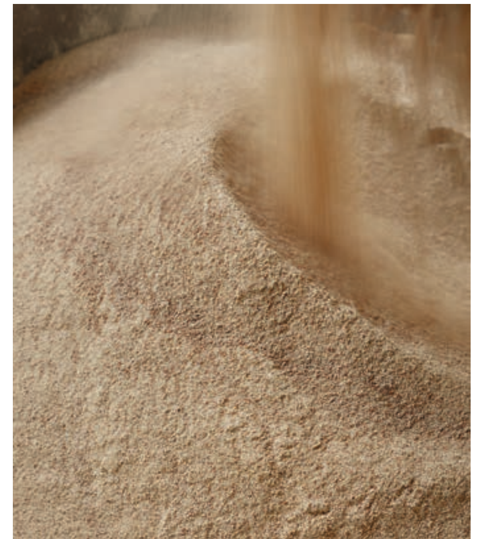
8. Calcium Carbonate Calcium carbonate, a by-product from the local drinking water industry, is added to the mix of polyolefin granules and pine rosin, and transformed to make the EcoBase backing for a new carpet tile.
