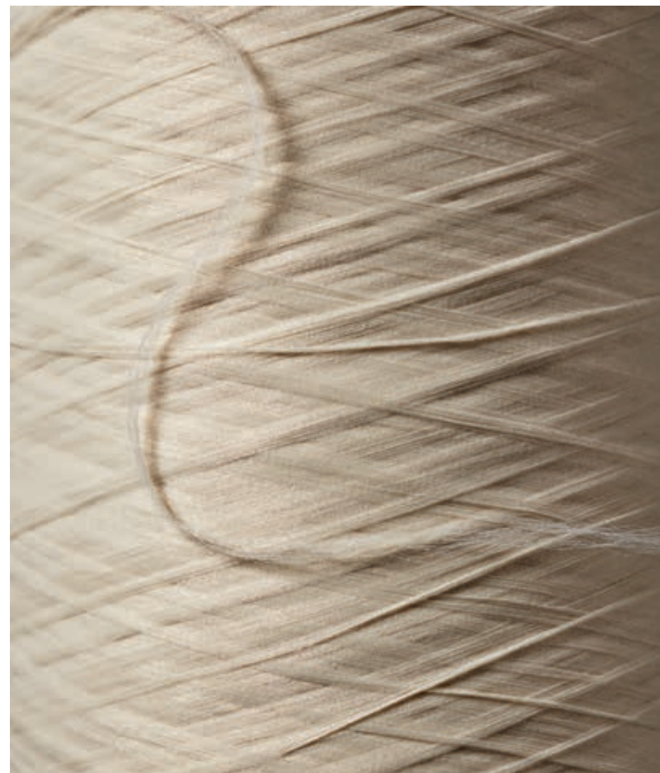
4. Polyamide 6 Nylon Yarn The PA6 nylon granules are then turned into new yarn, ready to produce the new generation of DESSO by Tarkett carpet tiles back in our factory.
