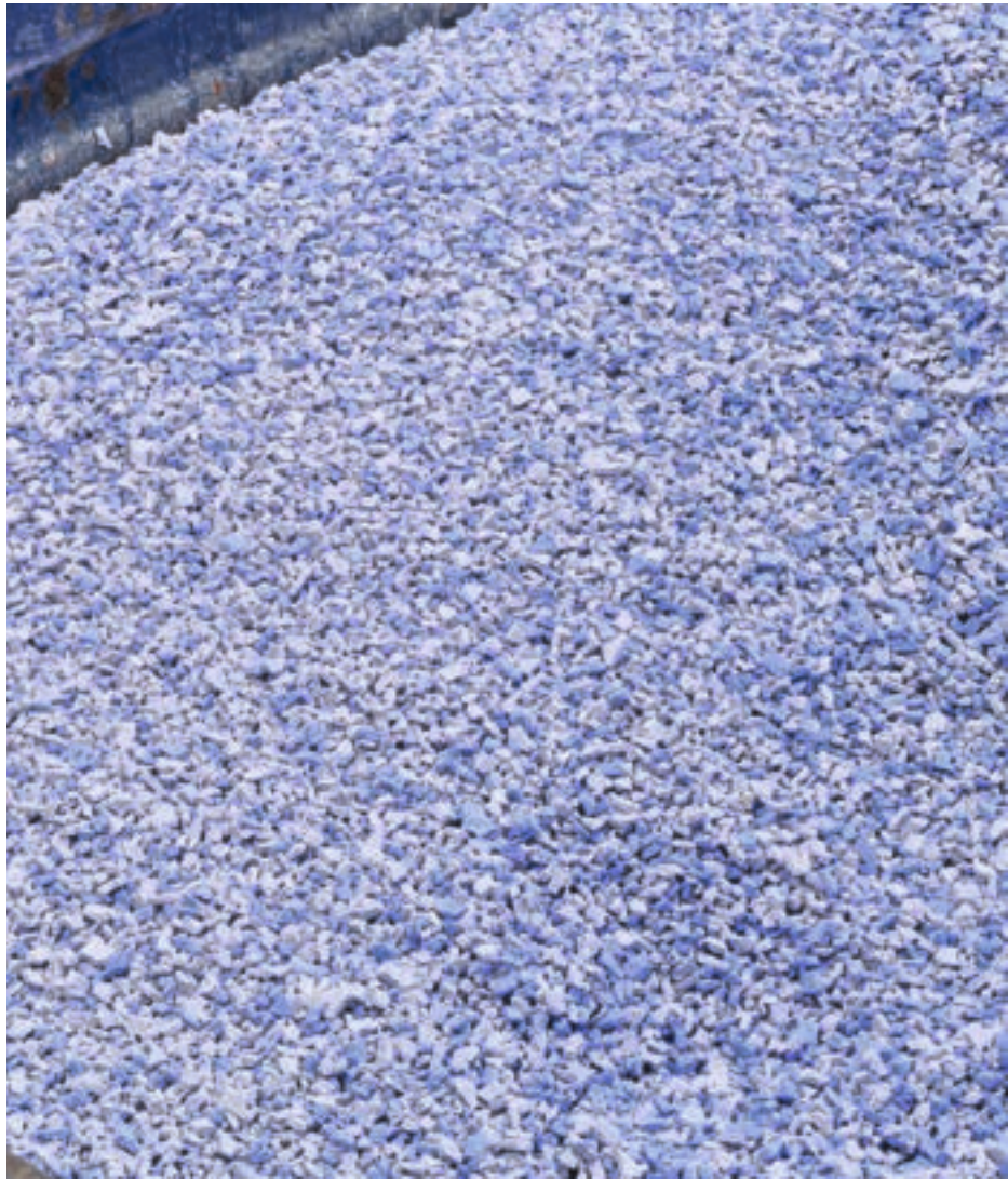
3. Recycled Granules At our recycling centre, the returned flooring is cleaned of glue and concrete before being crushed into granules.
