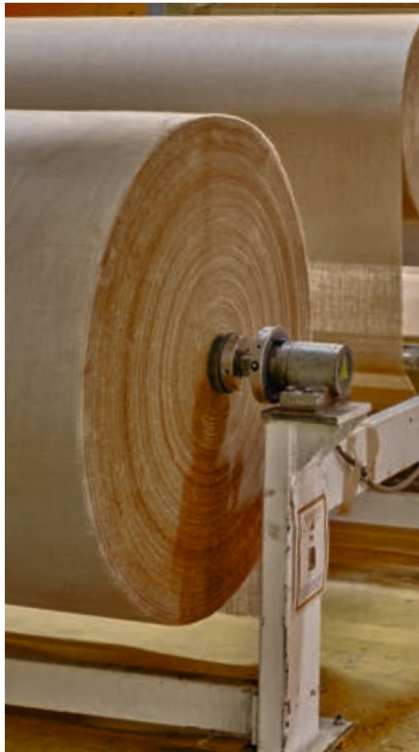
11. Jute Backing Jute, a carbon sequestering vegetable fibre, is woven into a strong textile to form the base for our linoleum flooring.
