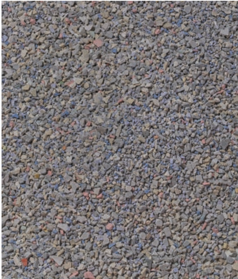
7. Finished Granules Once cooled, the semi-finished roll is crushed into granules and pressed to get the desired pattern and make a new generation of Tarkett's homogeneous vinyl flooring.
