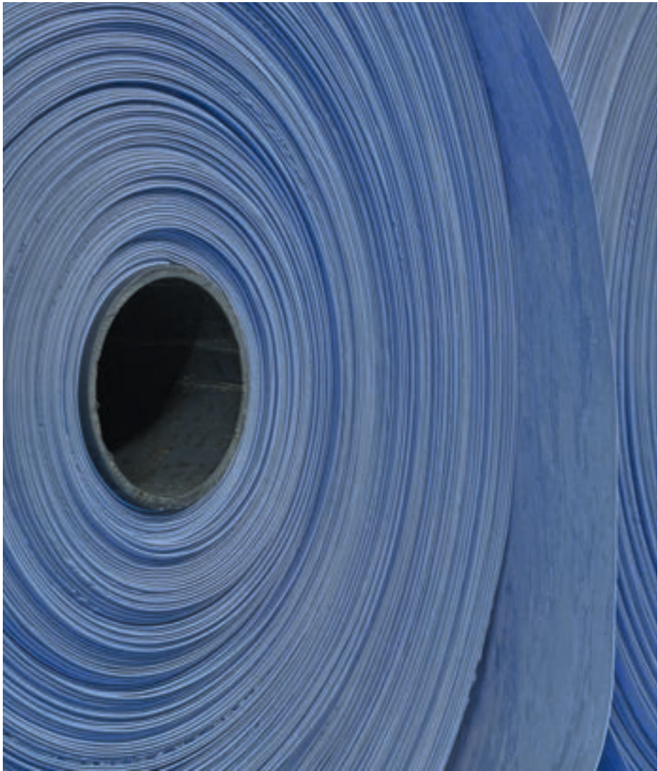
6. Semi-Finished Rolls Strands in three different colours are combined before being smoothed into a semi-finished roll.
