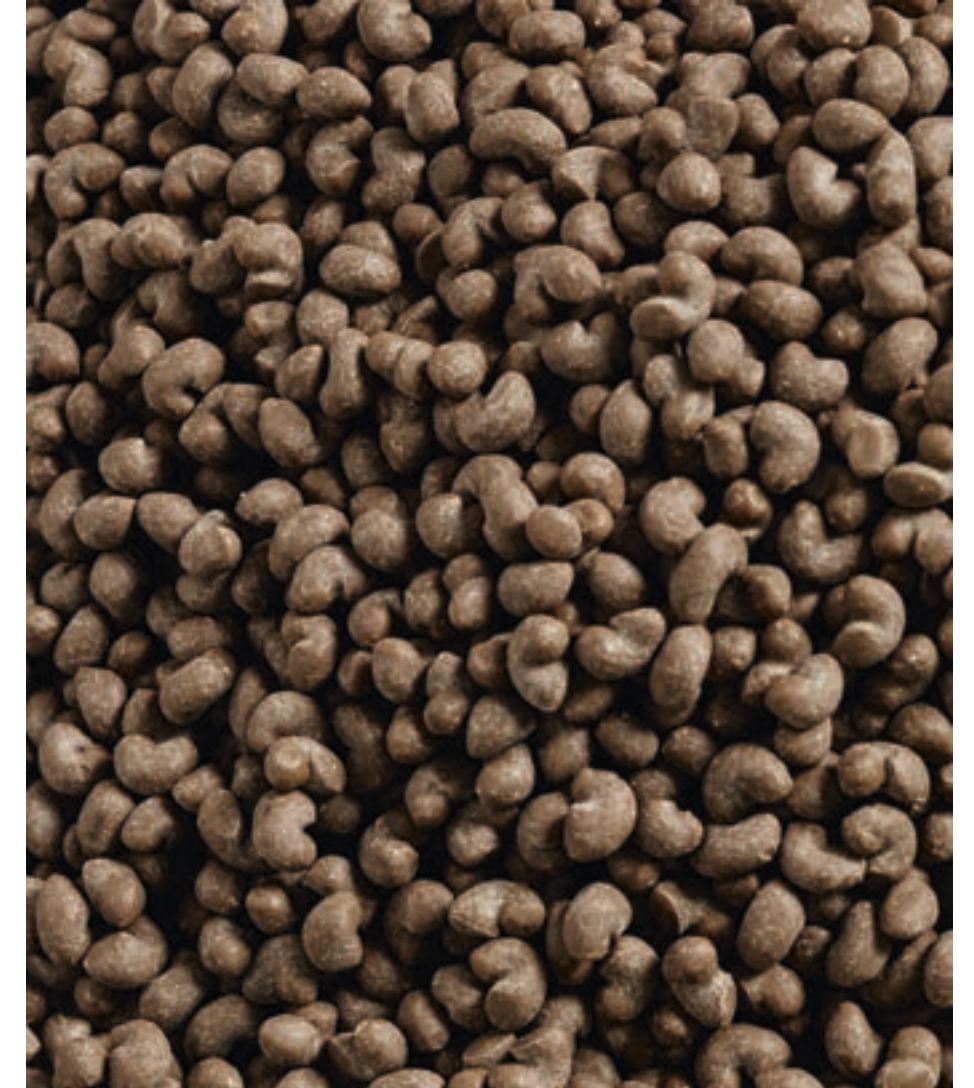
6. Polyolefin Granules Shredded EcoBase backing is transformed into polyolefin granules in a process that can be carried out over and over again, with no loss of quality.
