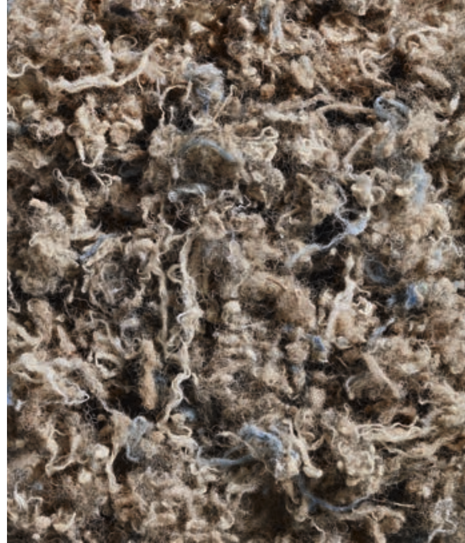
2. Reclaimed Polyamide 6 Yarn At our carpet recycling centre, the polyamide 6 yarn is separated from the EcoBase backing to be purified and regenerated.
