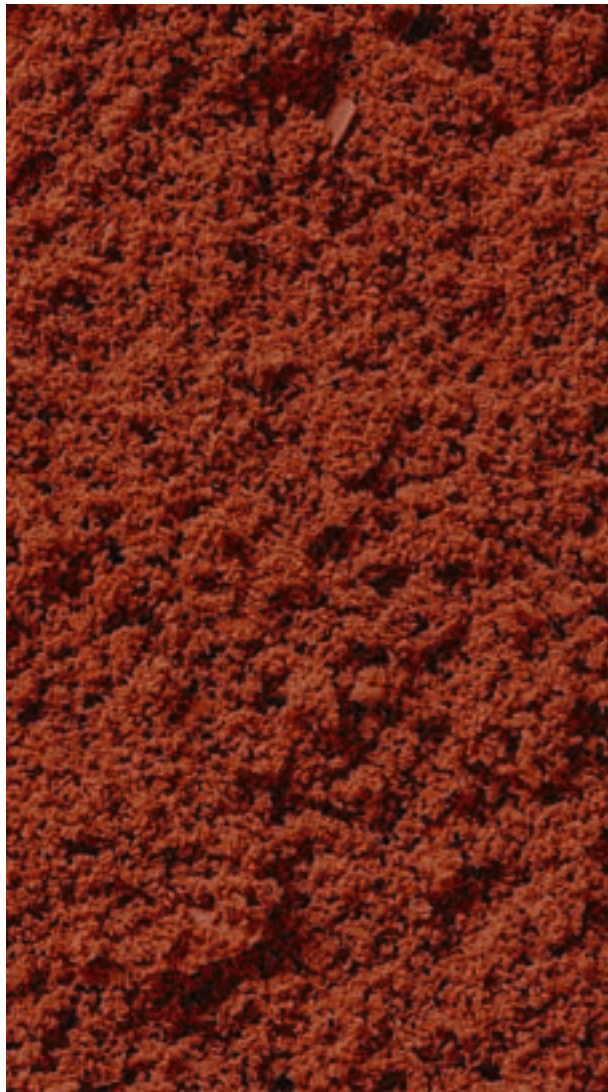
10. Linoleum Granules Linoleum cement is added to wood and cork flour, recycled linoleum powder and pigments to create linoleum granules.
