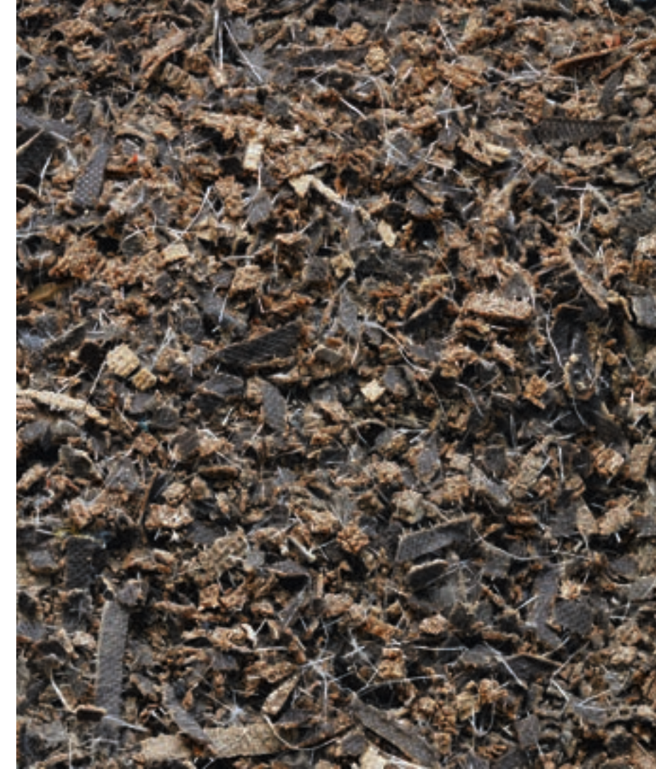
5. Shredded Backing At our carpet recycling centre, EcoBase backing is separated from the yarn, and shredded as we prepare it to be regenerated for circular reuse.
