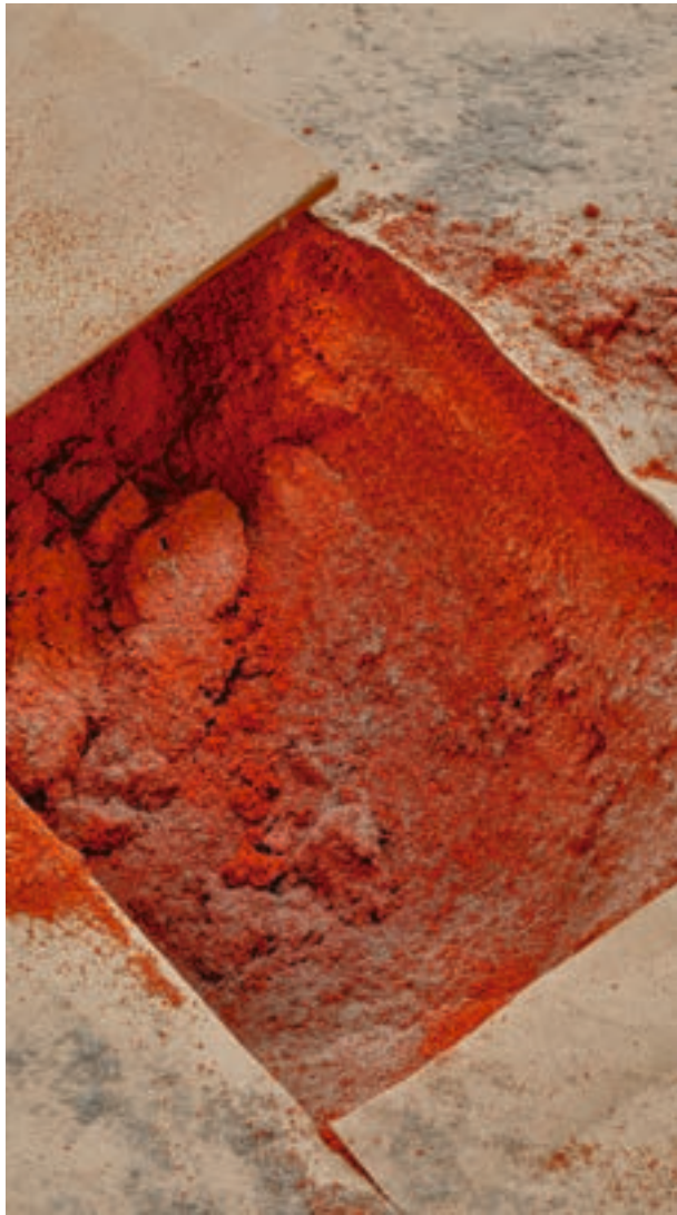
2. Recycled Linoleum Powder The shredded linoleum is ground into recycled linoleum powder, ready to re-enter production as a valuable raw material.
